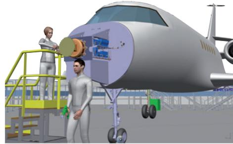
Validate maintenance costs and cycle times before operation with high-fidelity manikin-in-the-loop task simulation. Leverage full visibility of maintenance requirements to improve design-for-maintainability.
